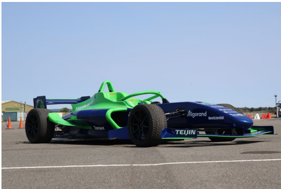
The world's first two-seater racing car featuring TENAX™ carbon fiber
