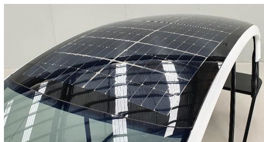
Left: New solar roof deployed in LS-EV prototype Right: Solar roof
