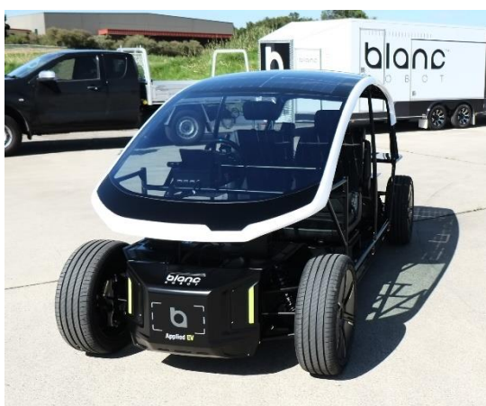
Left: New solar roof deployed in LS-EV prototype Right: Solar roof
