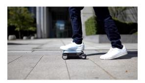
The *WALKCAR*<sup>®</sup>, which is small enough to be carried in a bag, measures just 21.5 cm by 34.6 cm, roughly the size of a 13-inch laptop computer, and weighs only 2.9 kg. The *WALKCAR*<sup>®</sup> can travel about 7 km at a maximum speed of 16 km/h on a single charge. Operated by simply shifting one's center of gravity, the APM requires neither a handle nor controller, and stops automatically as soon as the operator steps off.
