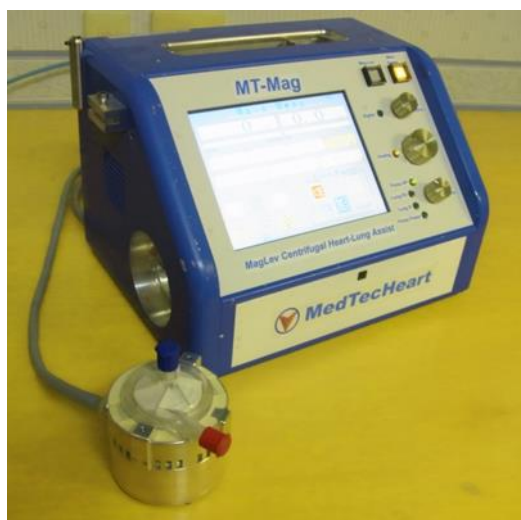
MT-Mag, MedTec-Magnetically levitated centrifugal ventricular assist device, under development in Japan and Europe
