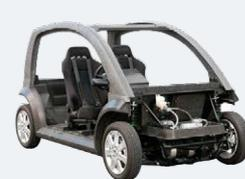
Thermoplastic CFRP concept car
