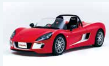
Tommykaira ZZ with polycarbonate-resin pillar-less front window
