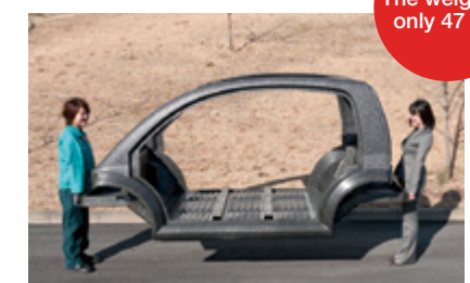
Concept car body-framework using thermoplastic CFRP
