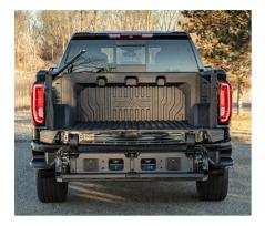
Teijin Group carbon fiber reinforced thermoplastic (CFRTP) products are used in General Motors pickup trucks.
