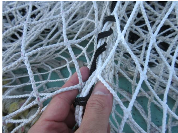
(left) MX-4 net showing almost no deterioration after approx. 300 uses and (right) unused knotless net
